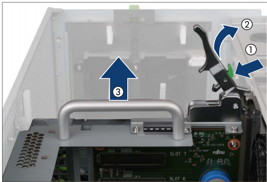
Figure 94: Removing the PCI Riser
